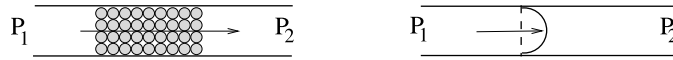
Fig. 4. Porous (left) versus elastic (right) medium. The total discharge Q of a fluid through a porous medium is proportional to the pressure drop P_2 - P_1 (Darcy's law). The deformation \bar{x} of an elastic membrane or spring is proportional to the applied force P_2 - P_1 (Hooke's law).
